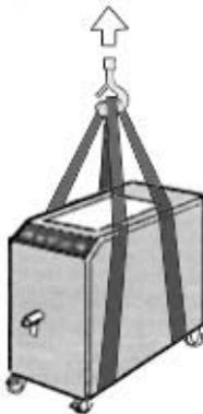
Lift machine with straps, keeping them near front and back wheels, as in the diagram the.
